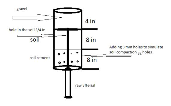
Injection speed: one revolution every half inch of height At a rate of 12 revolutions per minute
